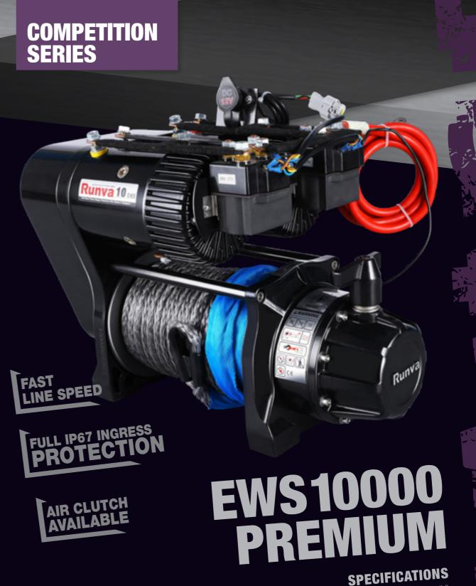
Rated Line Pull 10,000lb (4,536kg) I Motor Series Wound (12V) 2X 5.4kW/7.2HP(also available in 24V) Gear Ratio 108:1 (full steel gearing) | Clutch Stainless Steel rotary clutch. (optional extra air clutch available) Cable Type Synthetic Rope 10mm x 30m | Mounting Bolt Pattern 254mm x 114.3mm Overall Dimensions 479mm x 262mm x 355mm | Winch Body Colour Black Warranty See warranty document regarding competition usage
